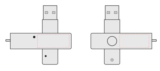
Front Laser Area : 27mm x 11mm Laser Engrave Back Laser Area : 25mm x 11mm Laser Engrave
